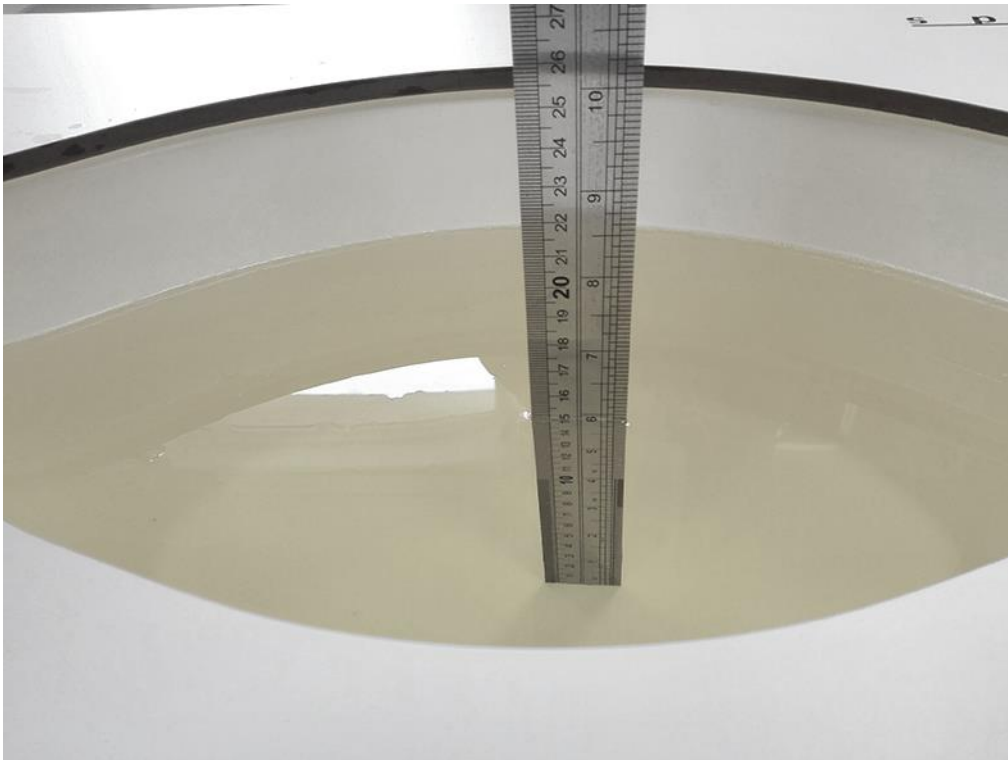
Liquid depth in the flat Phantom (2450 MHz, 15.3cm depth)
