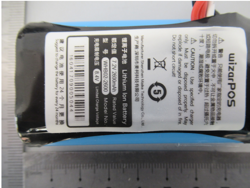
EUT – Battery Label View
