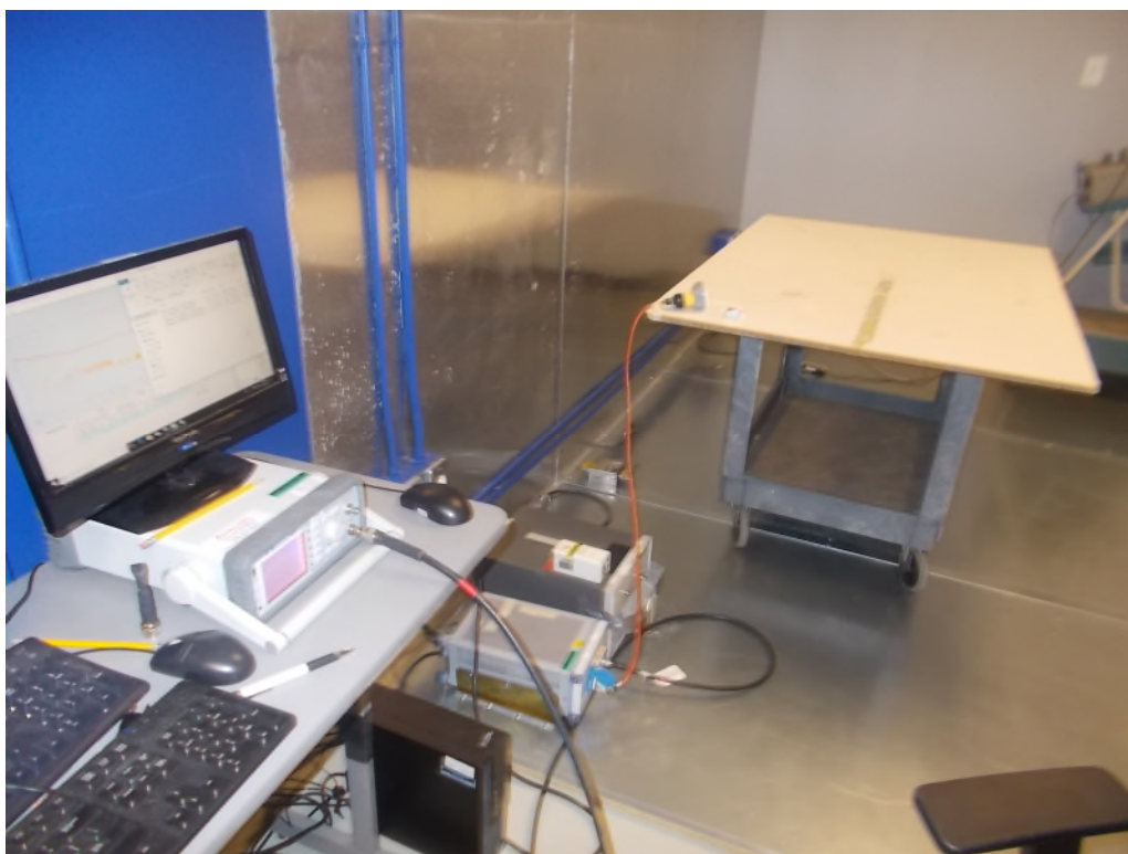
Figure 9: AC Power Line Conducted Emissions
