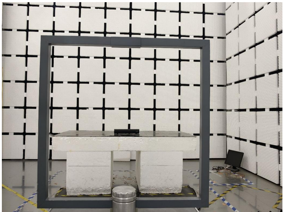
Radiation Emission Test Setup (Below 30MHz)
