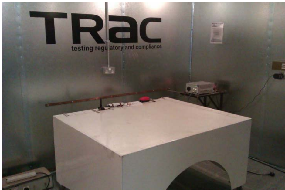
Test Setup AC powerline
