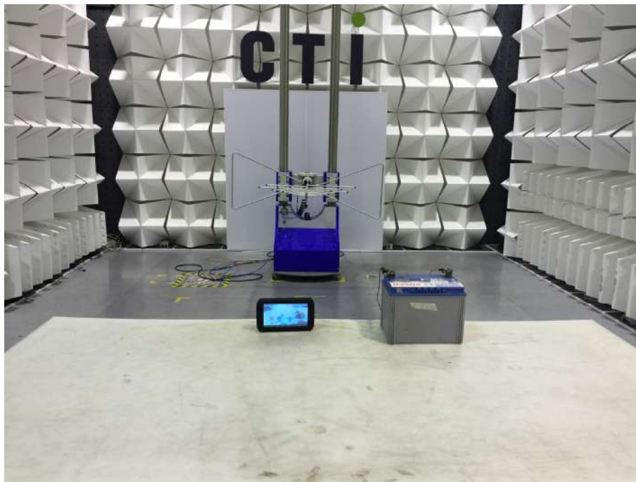
Radiated spurious emission Test Setup-1 (Below 1GHz)
