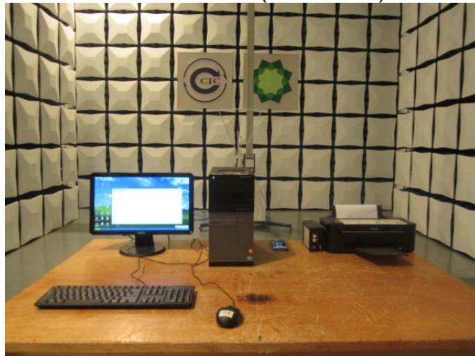
Radiated Emission (above 1GHz)
