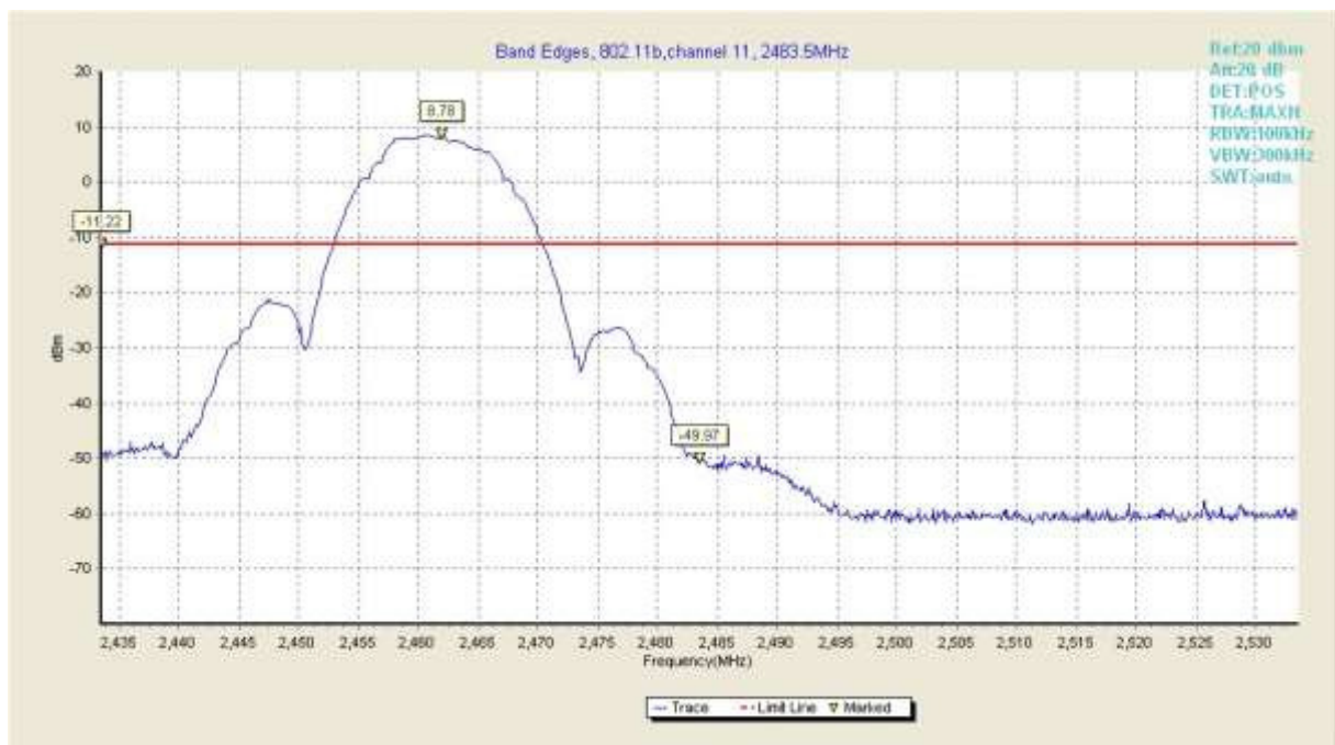
Fig26. Frequency Band Edges of 802.11b in channel 11,2483.5MHz
