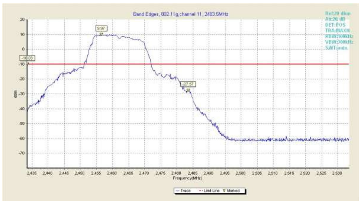
Fig28. Frequency Band Edges of 802.11g in channel 11,2483.5MHz
