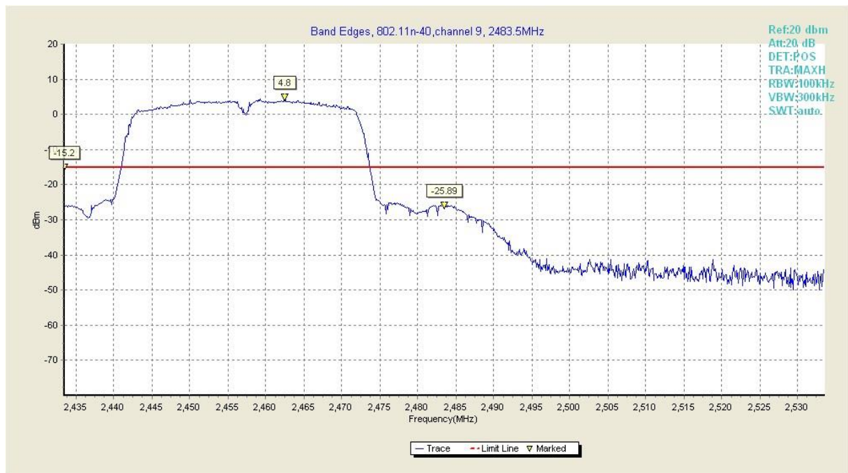
Fig32. Frequency Band Edges of 802.11n-40 in channel 11,2483.5MHz
