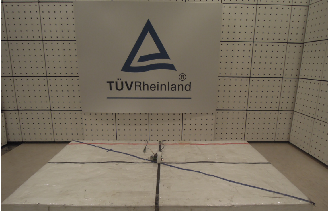
Photograph 2: Set-up for Spurious Emissions (Back View 1)
