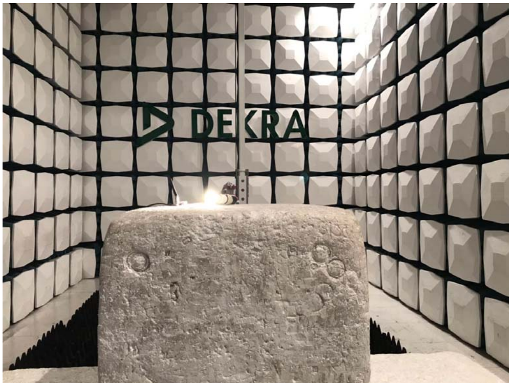
Description: Radiated Emission Test Setup for 1~18GHz
