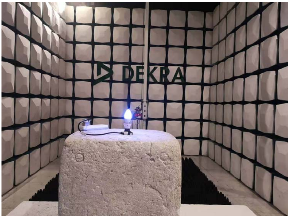
Description: Radiated Emission Test Setup for 1~18GHz
