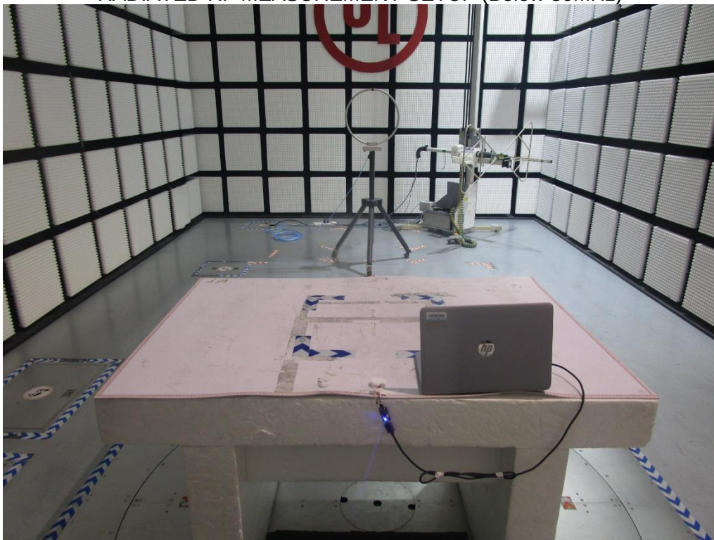
RADIATED RF MEASUREMENT SETUP (Below 30MHz)
