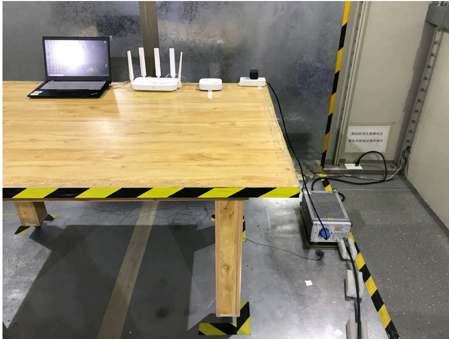
Conducted Emissions - Left View
