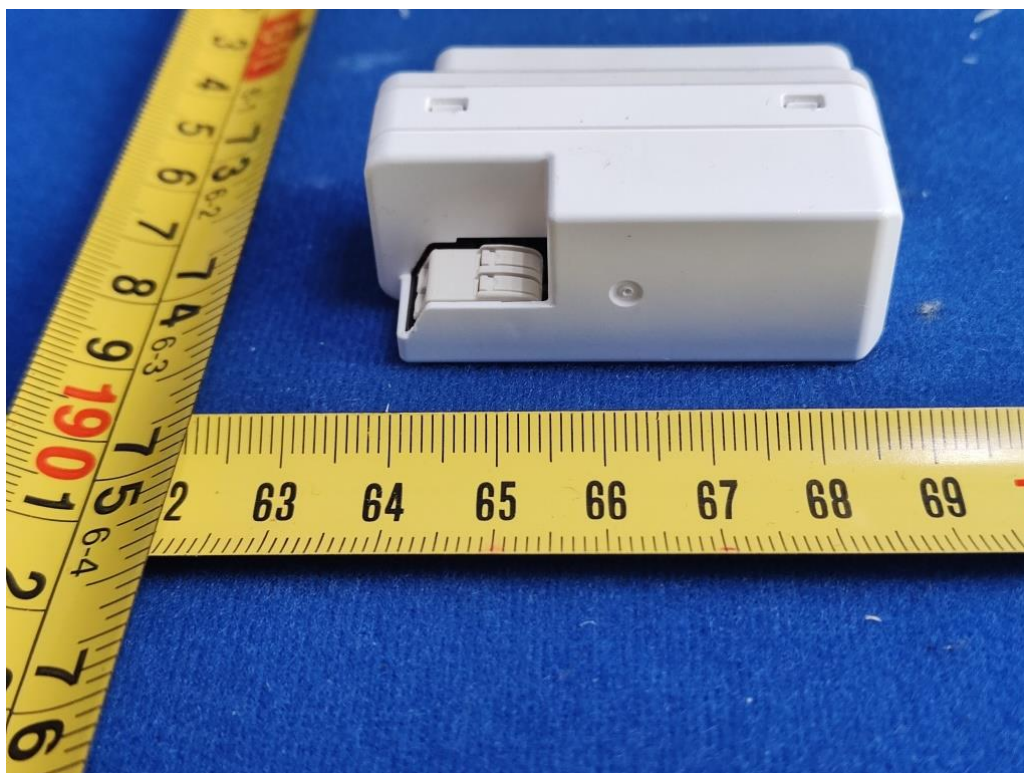
FIGURE 2 SENSOR (SC200B/02 SR SENSOR WH) BACK APPEARANCE
