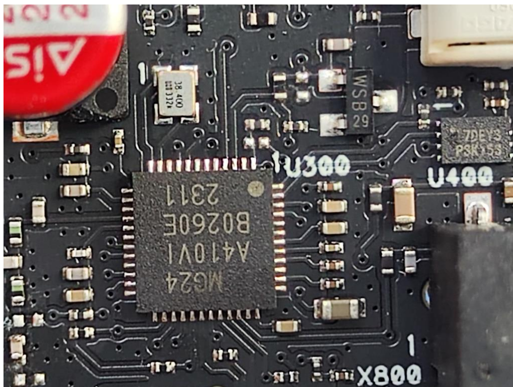
FIGURE 21 SENSOR (SC200B/02 SR SENSOR BL) CHIP & CRYSTAL
