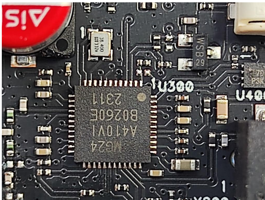
FIGURE 10 SENSOR (SC200B/02 SR SENSOR WH) CHIP & CRYSTAL
