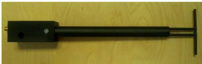
Figure 1 – MVG COMOSAR Validation Dipole
