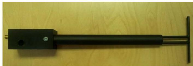
Figure 1 – MVG COMOSAR Validation Dipole
