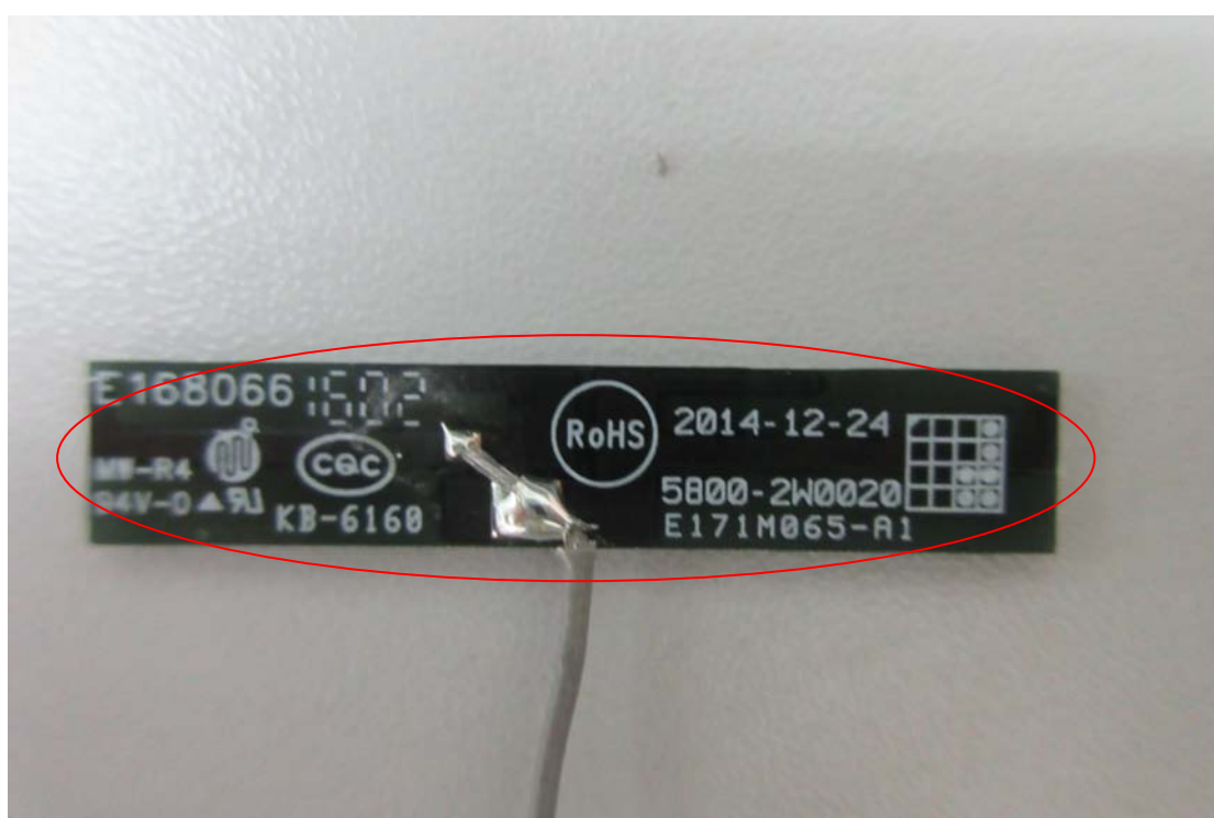
7. 5G antenna 1 view and 2.4G antenna 2 view
