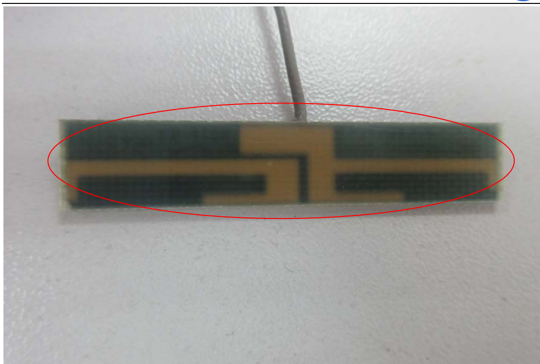
7. 5G antenna 1 view and 2.4G antenna 2 view
