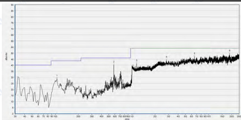
(Plot B.2: Antenna Horizontal, 30MHz to 25GHz)
