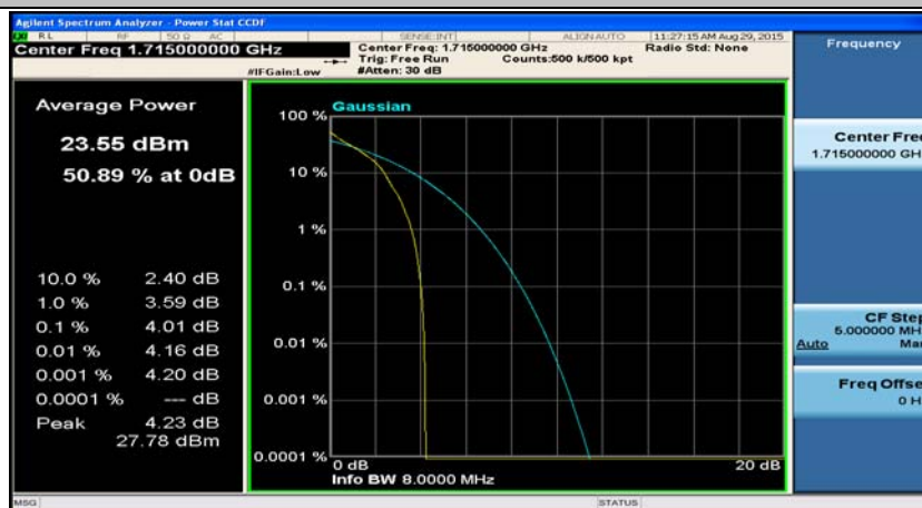
Channel Bandwidth: 10 MHz_LCH_QPSK_1RB#49
