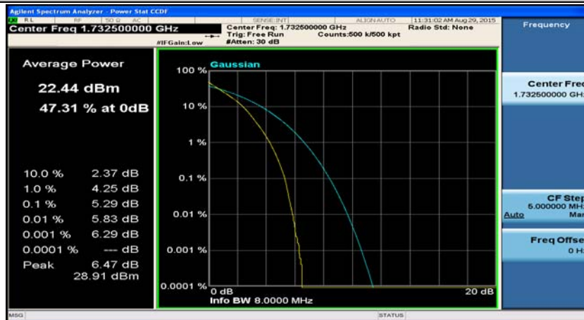
Channel Bandwidth: 10 MHz_MCH_QPSK_50RB#0
