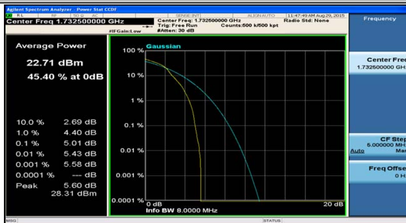
(Channel Bandwidth: 20 MHz)_MCH_16QAM_1RB#49
