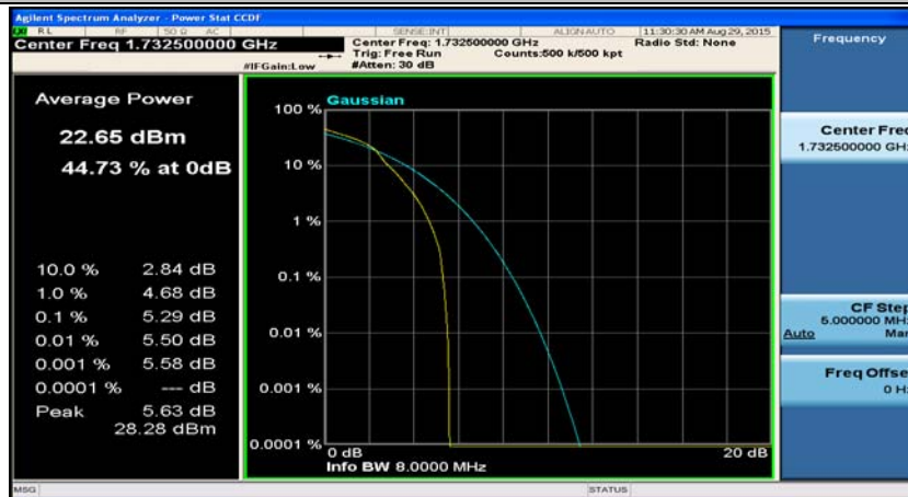
Channel Bandwidth: 10 MHz_MCH_16QAM_25RB#0
