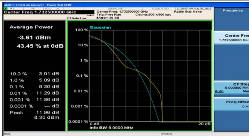
(Channel Bandwidth: 15 MHz)_MCH_16QAM_37RB#0
