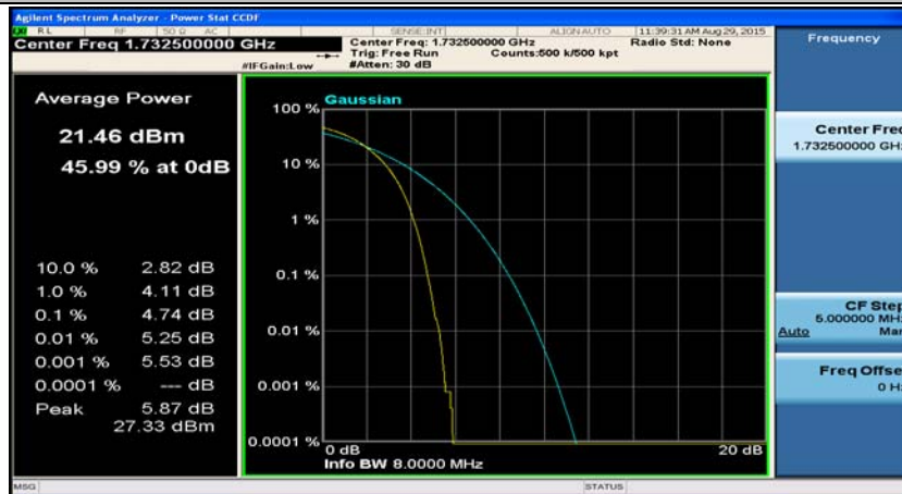
(Channel Bandwidth: 15 MHz)_MCH_QPSK_75RB#0
