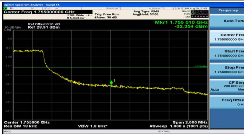
(Channel Bandwidth: 3 MHz)_HCH_QPSK_8RB#7
