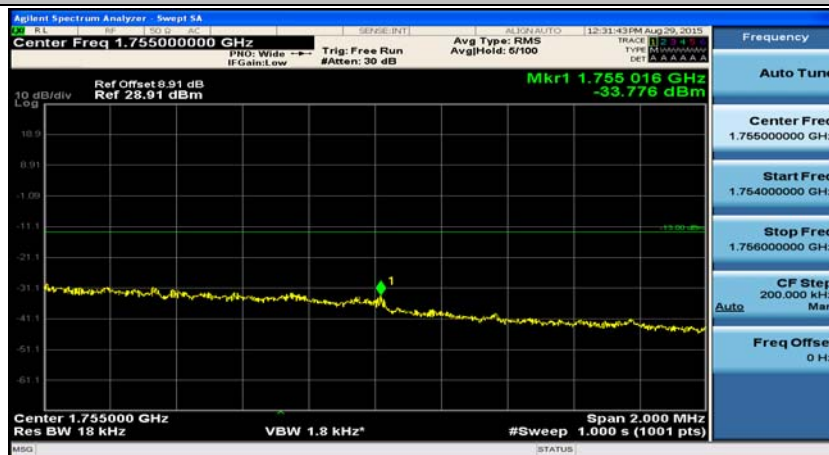
(Channel Bandwidth: 3 MHz)_HCH_QPSK_8RB#0
