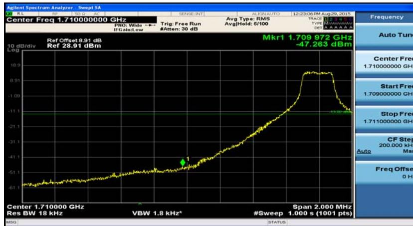
(Channel Bandwidth: 1.4 MHz)_LCH_16QAM_1RB#5
