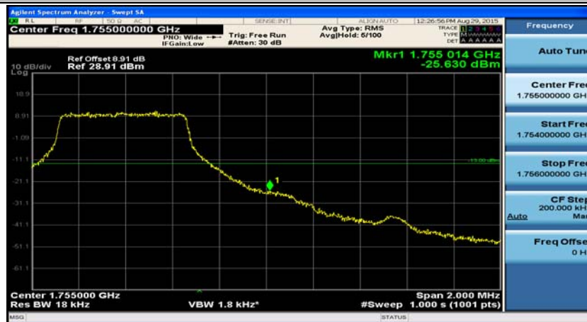
(Channel Bandwidth: 1.4 MHz)_HCH_16QAM_3RB#3
