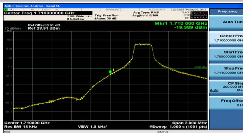
(Channel Bandwidth: 5 MHz)_LCH_16QAM_1RB#12
