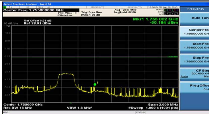
(Channel Bandwidth: 5 MHz)_HCH_QPSK_1RB#12
