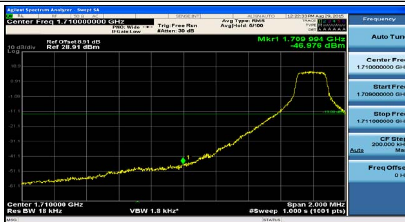
(Channel Bandwidth: 1.4 MHz)_LCH_QPSK_1RB#5
