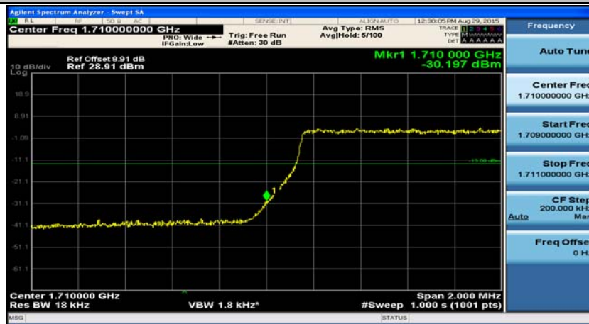
(Channel Bandwidth: 3 MHz)_LCH_QPSK_15RB#0
