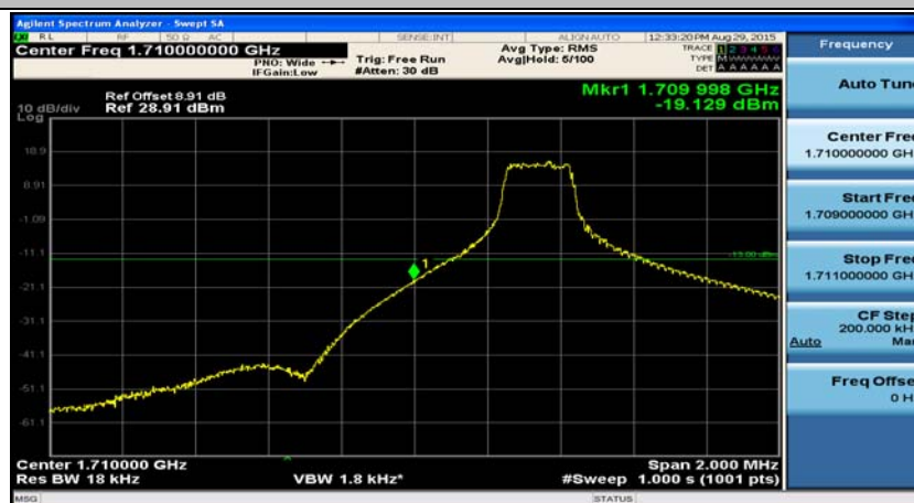
(Channel Bandwidth: 5 MHz)_LCH_QPSK_1RB#0
