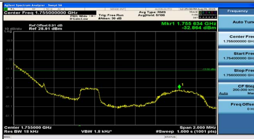
(Channel Bandwidth: 1.4 MHz)_HCH_QPSK_1RB#3
