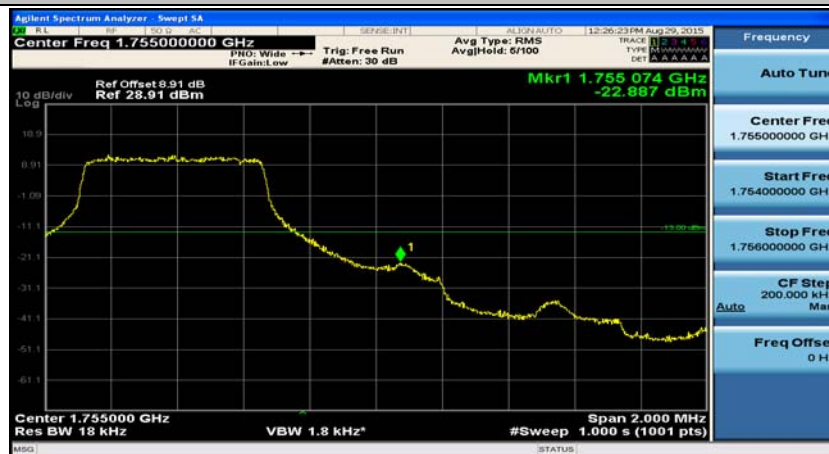
(Channel Bandwidth: 1.4 MHz)_HCH_QPSK_3RB#2
