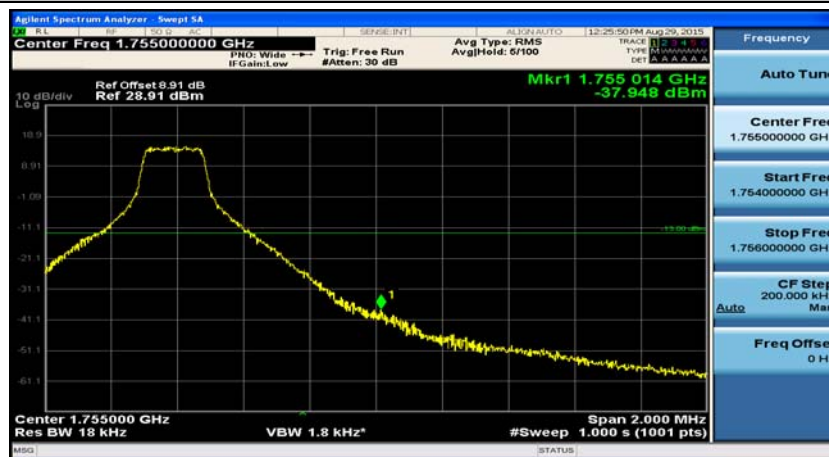
(Channel Bandwidth: 1.4 MHz)_HCH_16QAM_1RB#5
