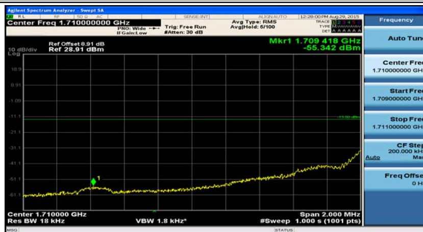
(Channel Bandwidth: 3 MHz)_LCH_QPSK_1RB#7
