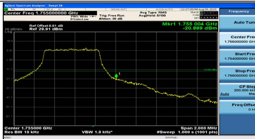
(Channel Bandwidth: 1.4 MHz)_HCH_16QAM_3RB#3
