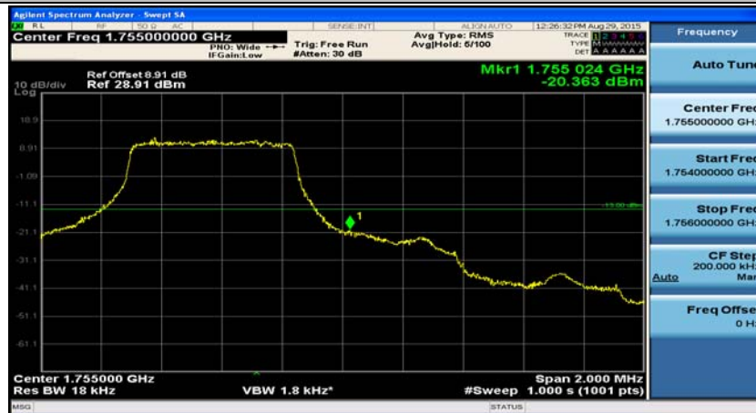
(Channel Bandwidth: 1.4 MHz)_HCH_QPSK_6RB#0
