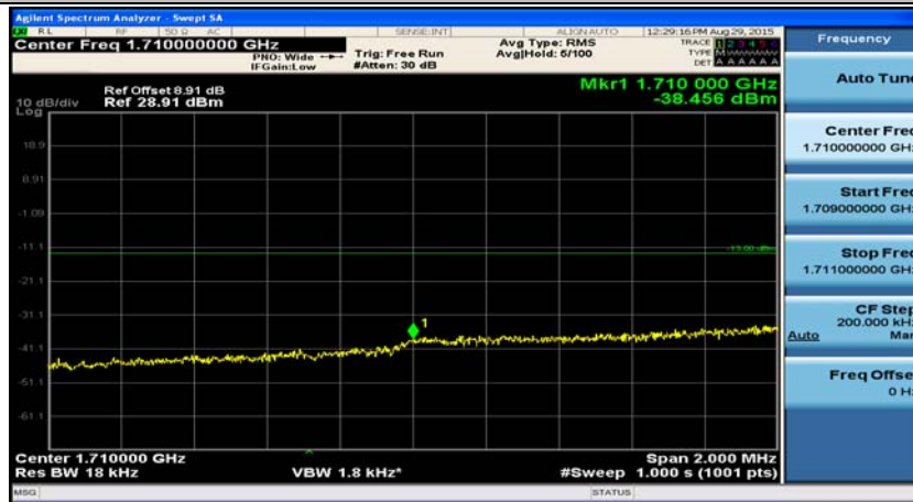
(Channel Bandwidth: 3 MHz)_LCH_QPSK_15RB#0
