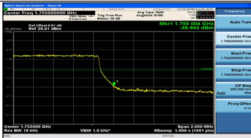
(Channel Bandwidth: 3 MHz)_HCH_QPSK_15RB#0
