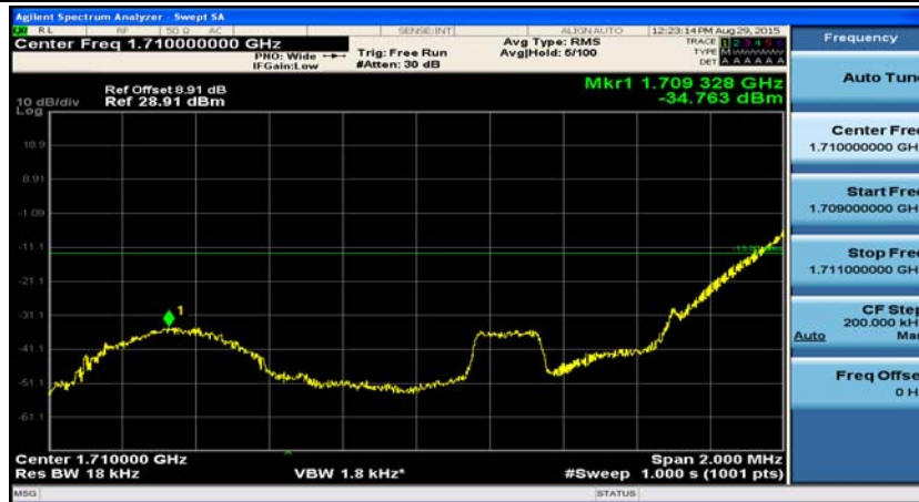
(Channel Bandwidth: 1.4 MHz)_LCH_16QAM_3RB#0
