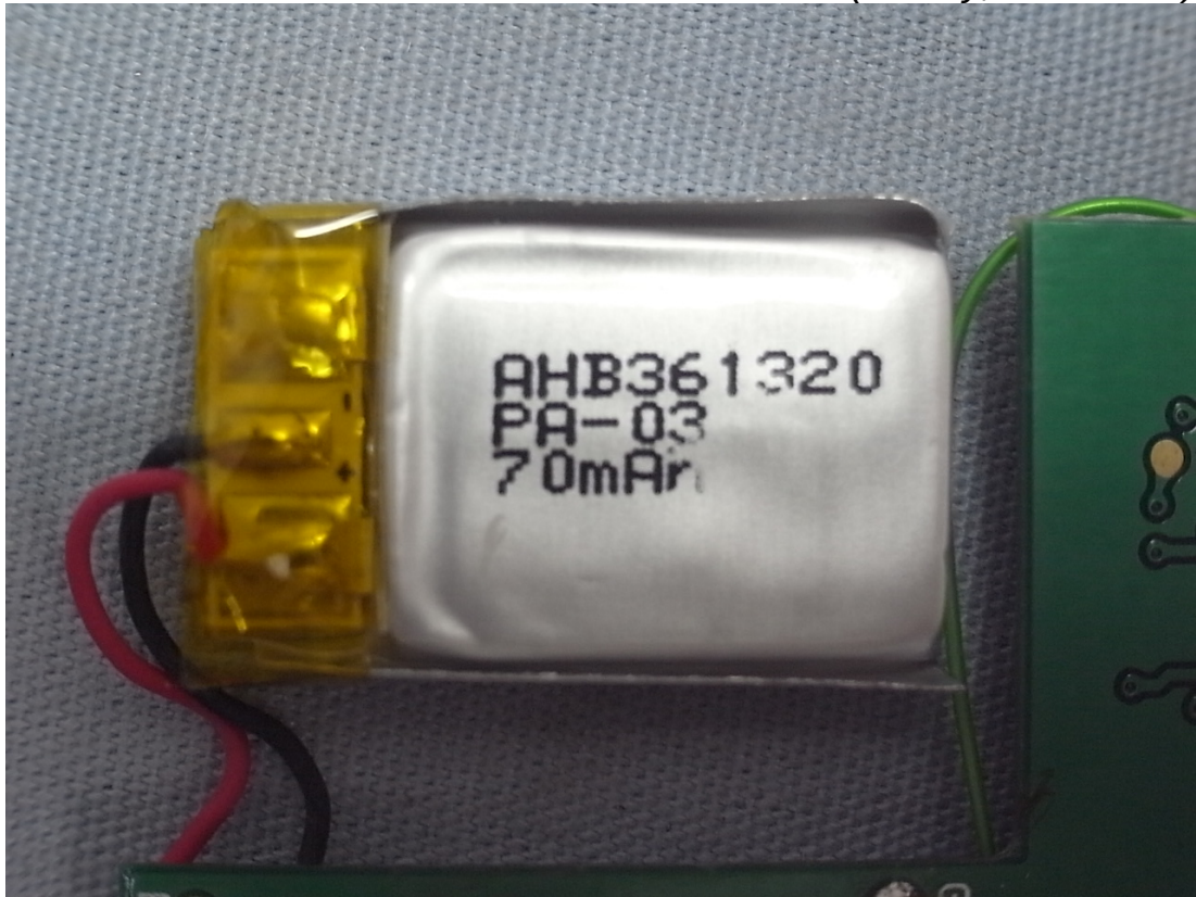
Figure 11 Internal View (Battery, Front View)
