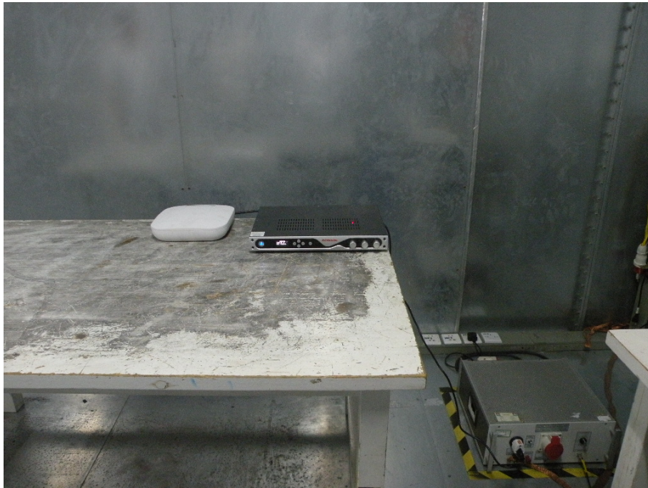
Photos of Conducted Emission test
