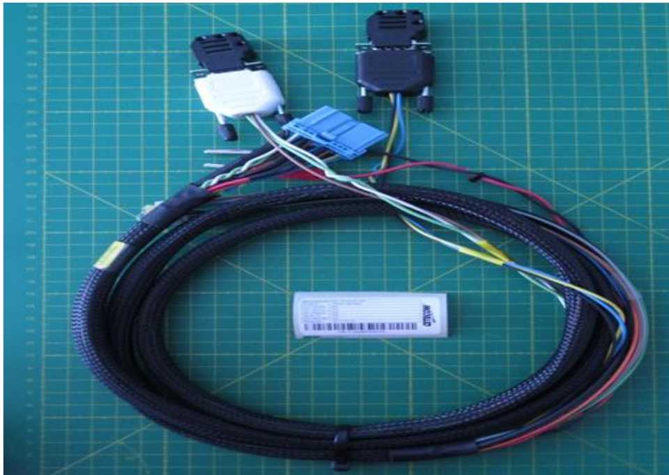
Photograph 8: AE1 – Cable Harness
