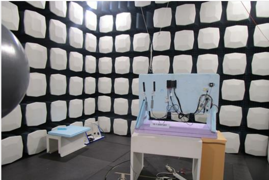
Photograph 1: EUT Test Setup in the anechoic chamber, Radiated interference field strength
