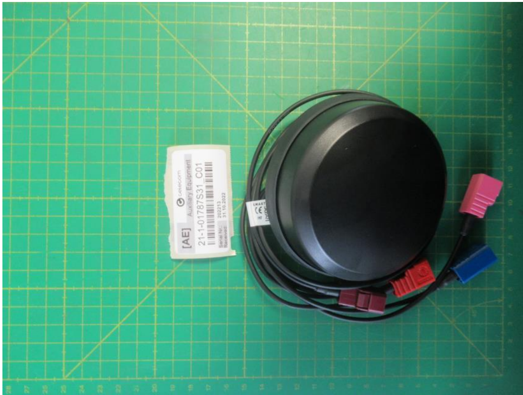
Fig. Ext.: 5 : Ext. - Front Cellular, GNSS and WIFI Antenna
