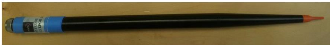
Figure 1 – MVG COMOSAR Dosimetric E field Dipole
