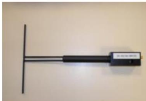
Figure 1 – Satimo COMOSAR Validation Dipole
