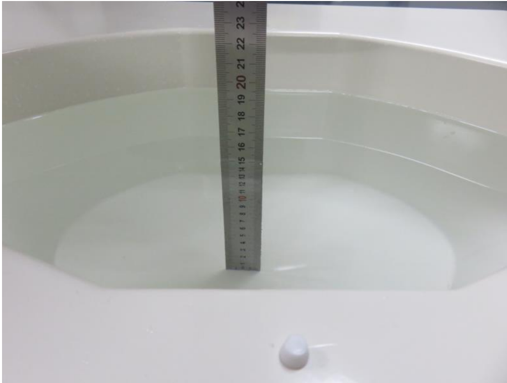
Photograph of the depth in the Body Phantom (750MHz, 15.5cm depth)
