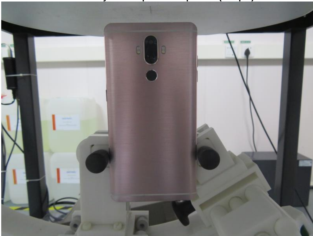
10mm body-worn Top Side Setup Photo (hotspot)
