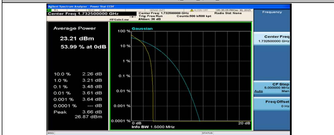
(Channel Bandwidth: 1.4 MHz)_MCH_QPSK_1RB#3
