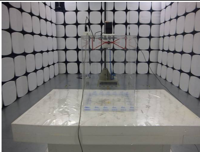
Radiated Spurious Emissions Test Setup Below 1GHz
