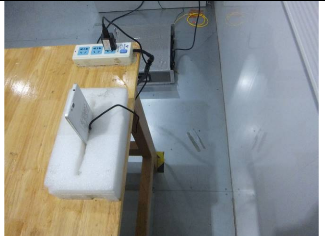
Conducted Emissions Test Setup Side View
