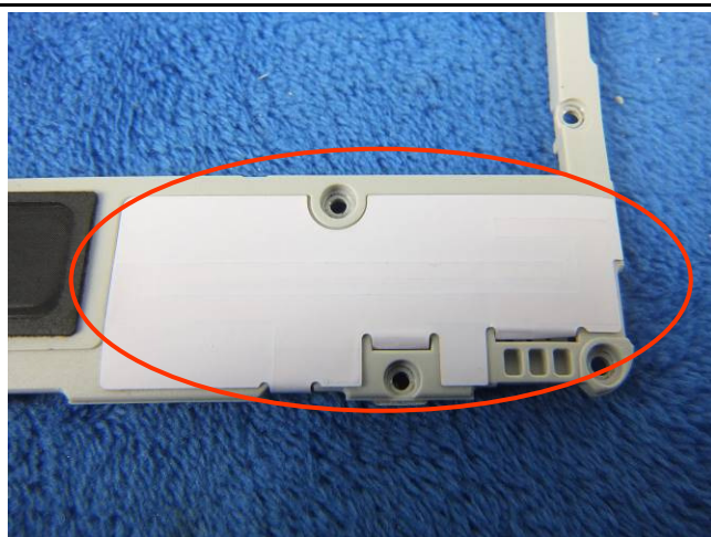
GSM/PCS/UMTS-FDD - Antenna View
