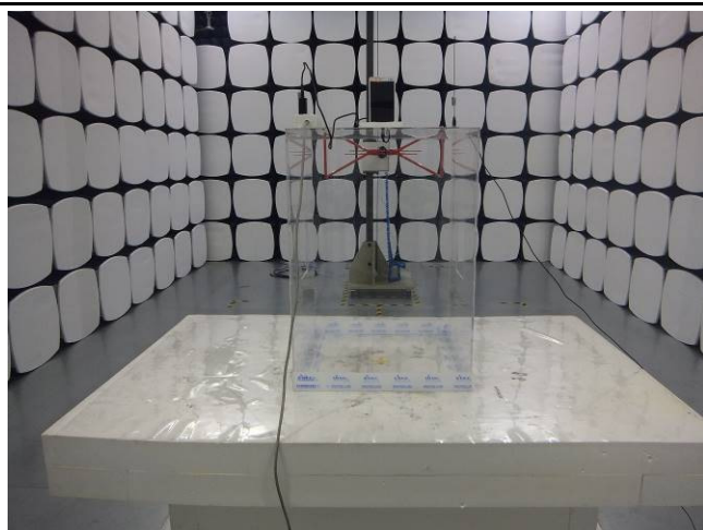
Radiated Spurious Emissions Test Setup Below 1GHz
