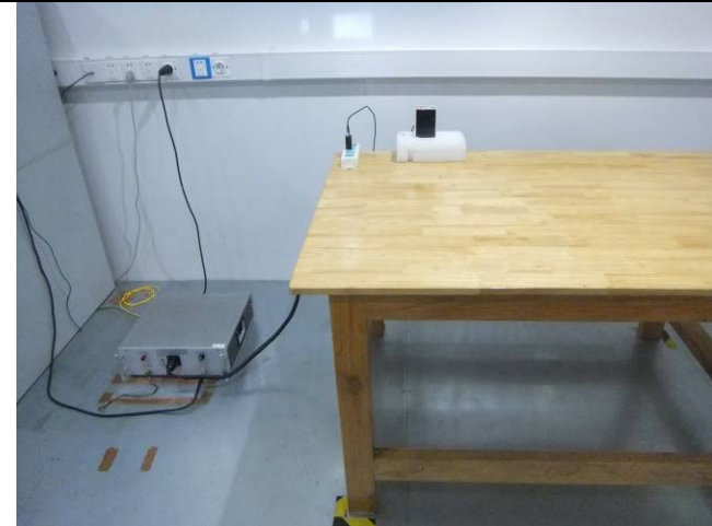
Conducted Emissions Test Setup Front View
