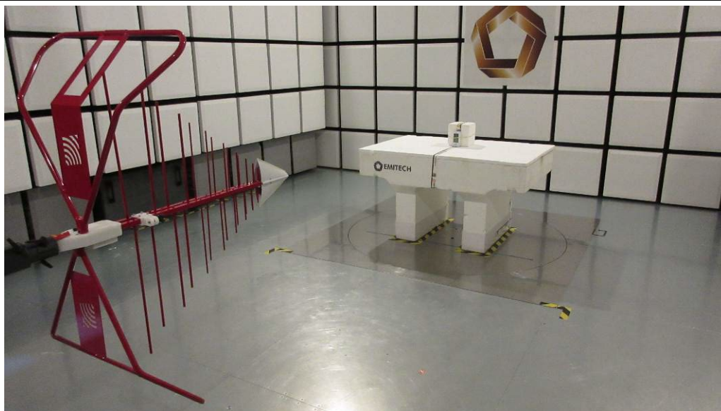
TEST SETUP PHOTO(S) – 30MHZ TO 1GHZ
