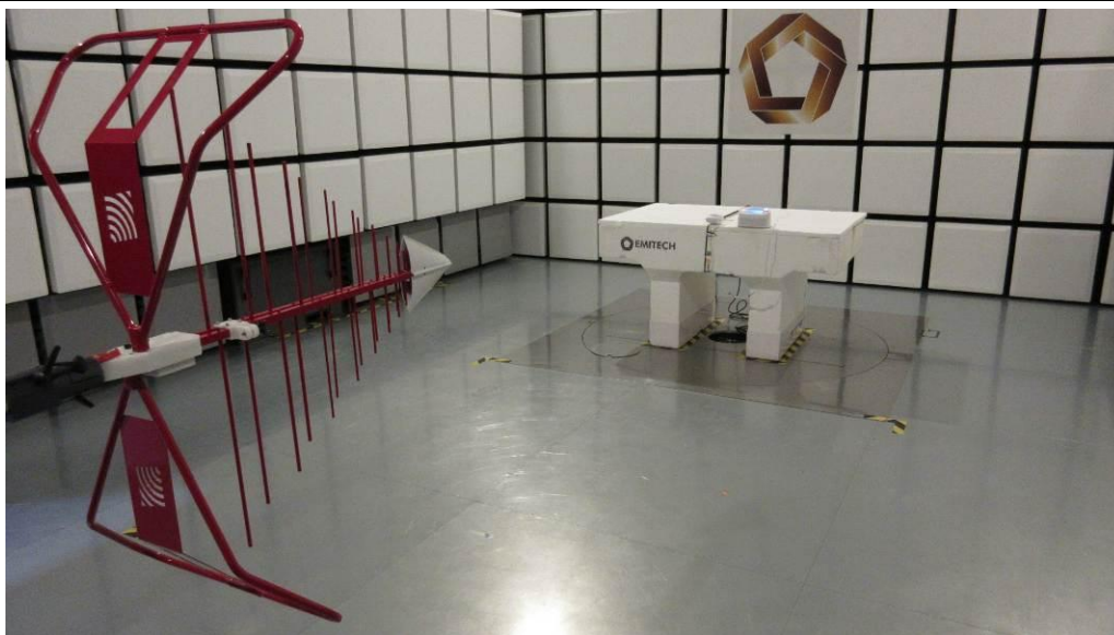
TEST SETUP PHOTO(S) - 30 MHz TO 1 GHz
