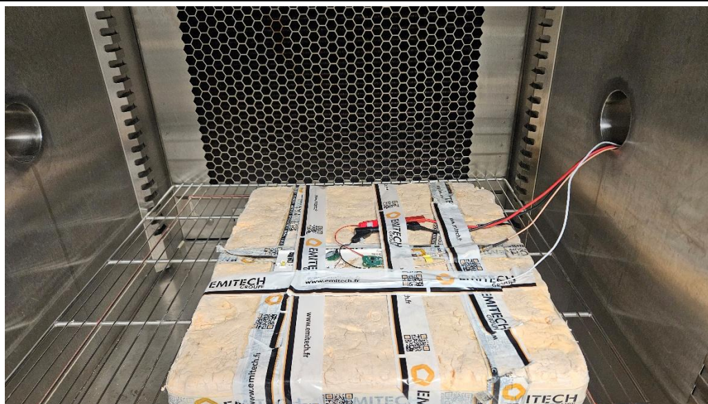
TEST SETUP PHOTO(S) - LOW CHANNEL / 25°C / 3.00Vdc
