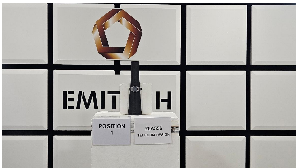
TEST SETUP PHOTO(S) - RADIATED MEASUREMENT – WITH PHANTOM ARM (STANDARD)
