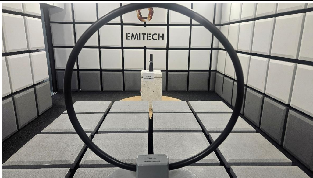
TEST SETUP PHOTO(S) - RADIATED MEASUREMENT – 9kHz TO 30MHz
