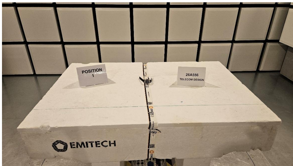
TEST SETUP PHOTO(S) - RADIATED MEASUREMENT – WITHOUT PHANTOM ARM (LP)
