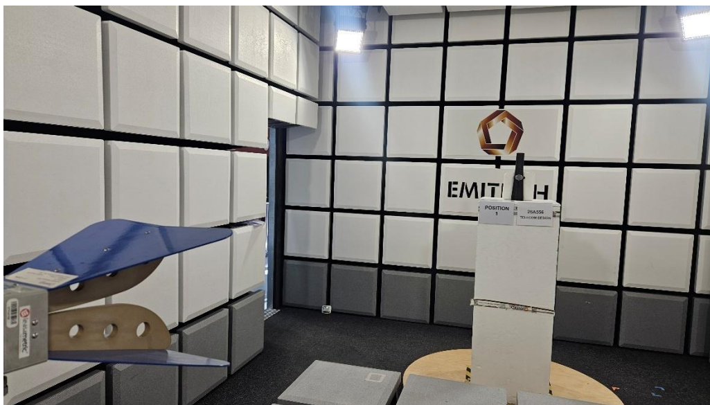
TEST SETUP PHOTO(S) - RADIATED MEASUREMENT – FOR FREQ &gt;1GHz
