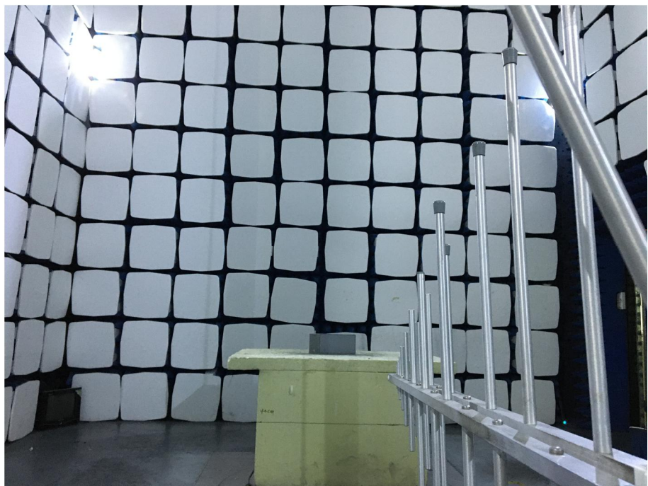
Radiation Emission Test Setup (30MHz to 1GHz)
