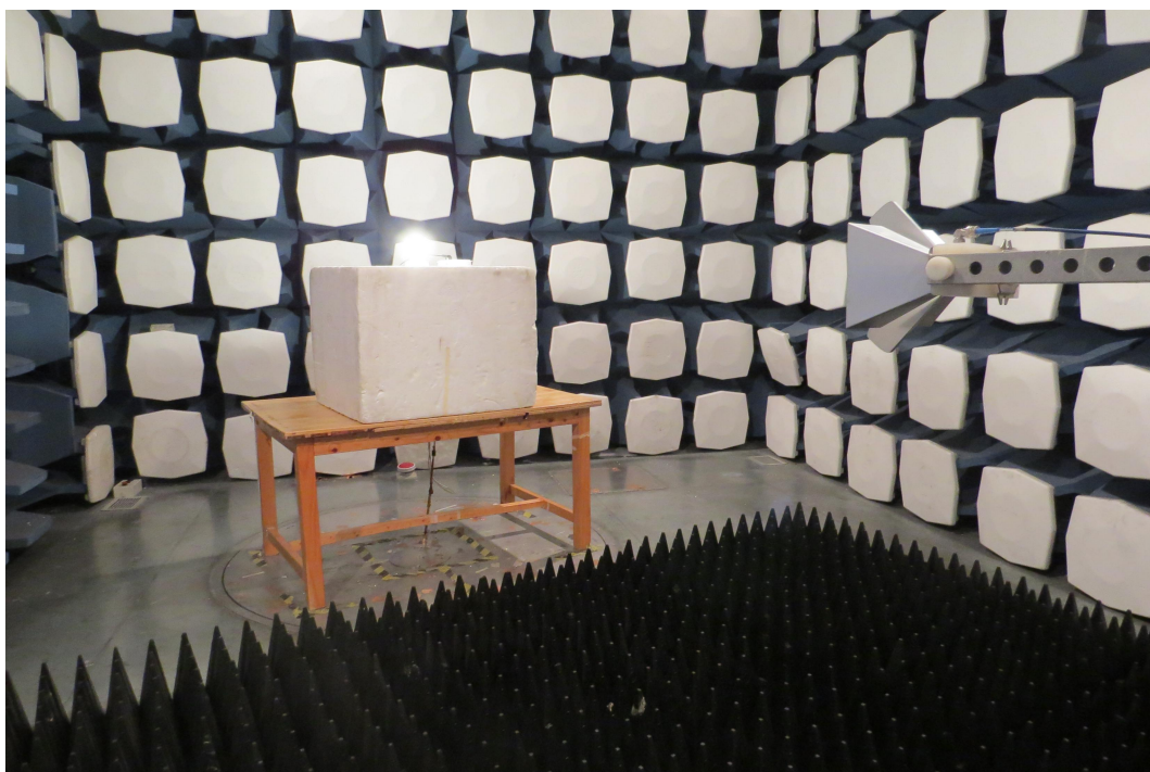
Picture 2 Radiated Emission Test Setup
