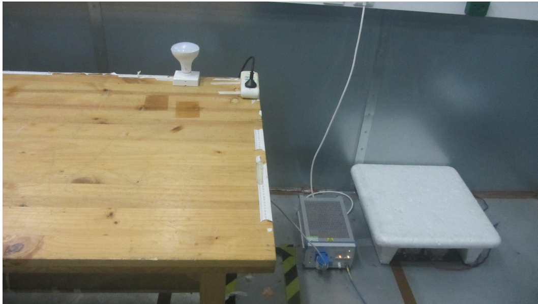
Picture 3 Conducted Emission Test Setup
