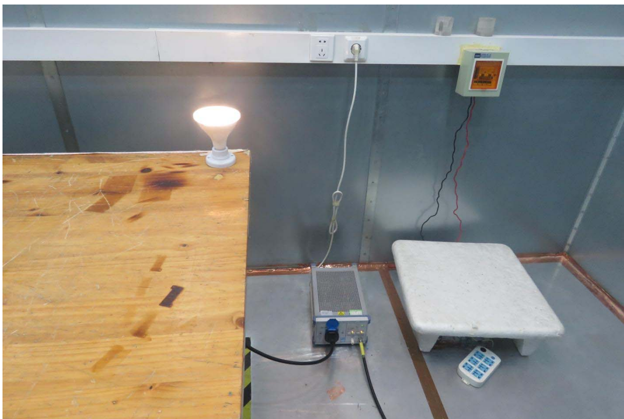
Picture 2: Conducted Emissions Test Setup
