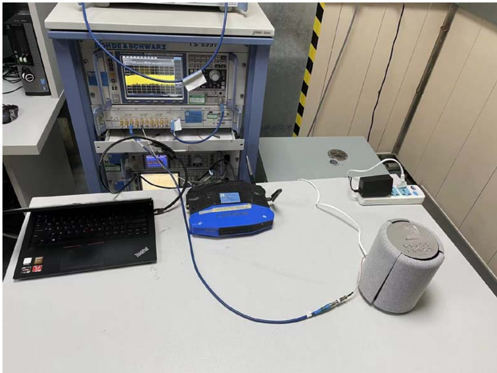
Dynamic Frequency Selection test
