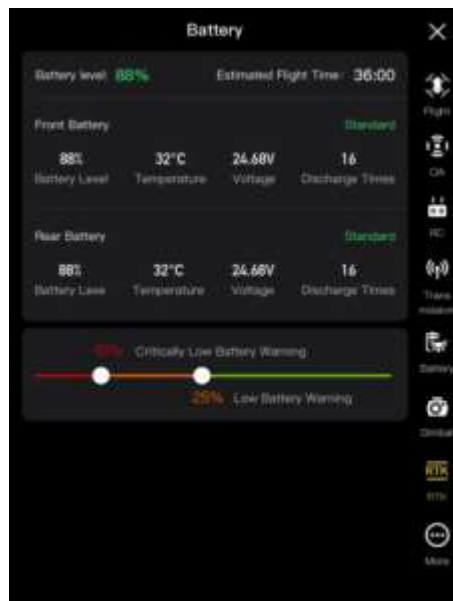
Fig 6-8 "Battery Information" Interface
