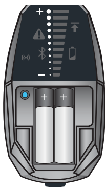
Figure 17. Battery compartment and battery placement
