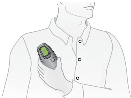
Figure 12. Correct positioning of sleep remote over generator
