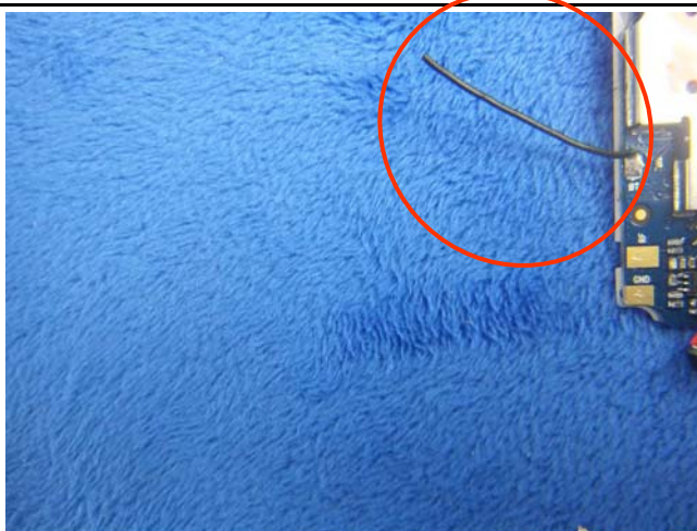
BT - Antenna View
