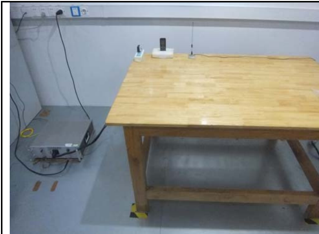
Conducted Emissions Test Setup Front View
