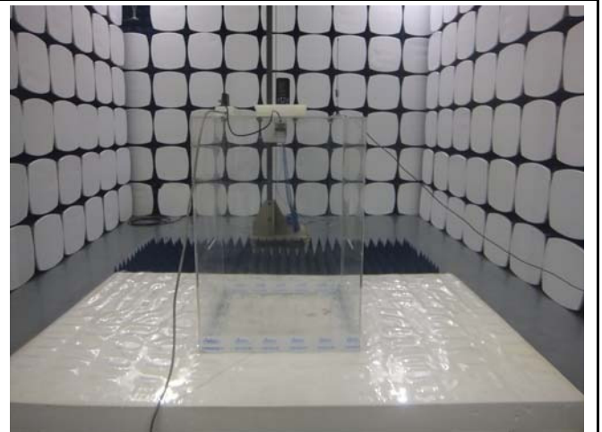
Radiated Spurious Emissions Test Setup Above 1GHz
