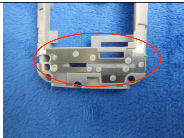
GSM/PCS Antenna View
