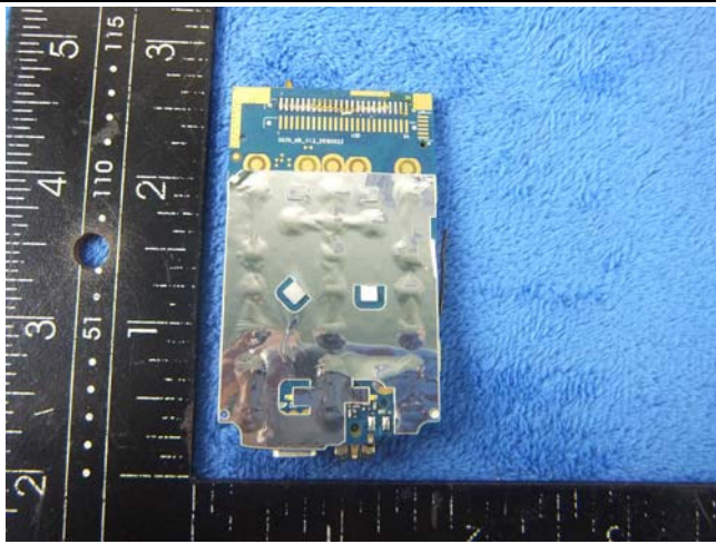
Mainboard with Shielding - Rear View
