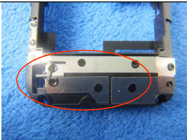
GSM/PCS Antenna View
