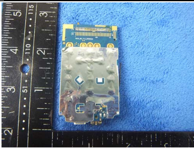
Mainboard with Shielding - Rear View
