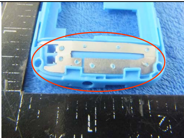
GSM/PCS Antenna View
